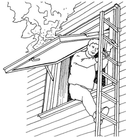
Fig. 1 MODUM Original Fire Escape Ladders in use during escape.
